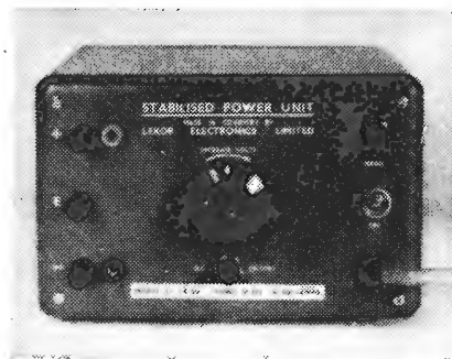
Lexor power unit. Sockets for external voltmeter are near terminals.
